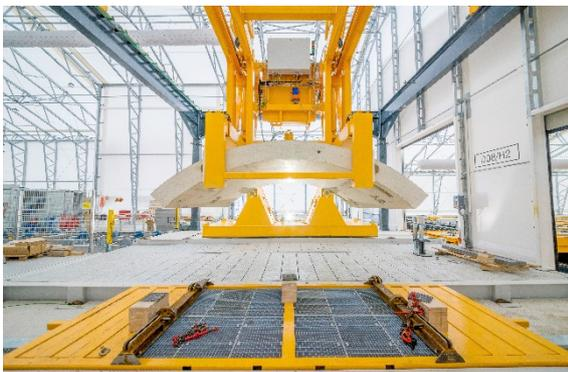
The heart of the mobile fabrication: The CNC concrete milling system.
