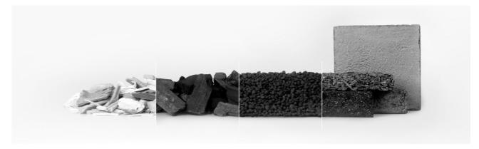
Biomass residues are processed into CO2-reducing, technical biocarbon materials, which are ultimately used as building materials and in this way bind carbon in buildings, streets and green spaces in the long term.
