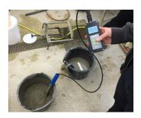
The easy and fast check of the correct water content can exclude later problems to the building. The previous kiln-drying-
