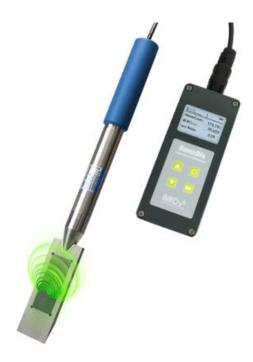
The figure shows the SONO-WZ probe. Green shows the radar wave which travels nearly with light speed along the probes surface. Similar to a CT, the fresh concrete is measured disc-shaped and layer by layer. The travel time which is measured with an accuracy of one picosecond (on the 12<sup>th</sup> decimal place) corresponds to the moisture content.
