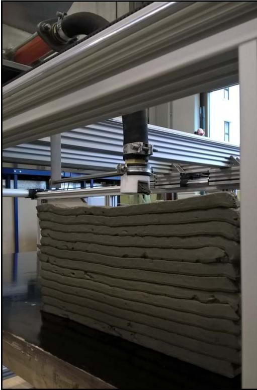
Fig 2: Laboratory tests for 3D concrete printing
